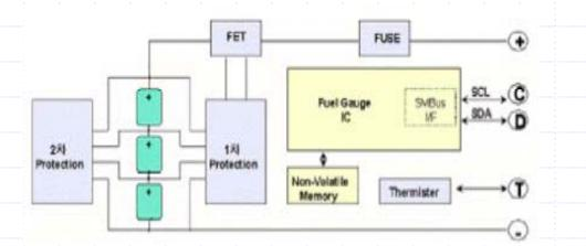
Fuel Gauge Circuit -- Monitoring power condition of battery and transmits data to host (notebook, PC, video camera, or cell phone) Protection Circuit -- Providing primary and secondary protection functions to battery Code Identification,
