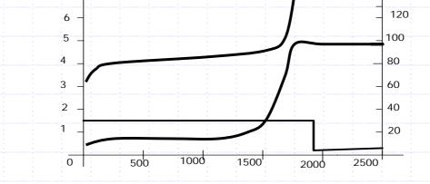
\*PPTC tracks cell temperature until cell reaches 80degC at which PPTC trips and limits current
