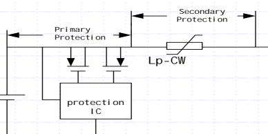
Voltage sensing IC controls dual-FET to provide primary overcharge protection; PPTC gives secondary overcharge and short-circuit protection
