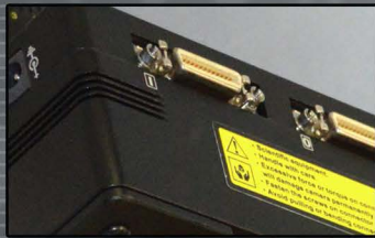
Camera Link interface: An industrially proven standard for high speed image data transmission. GigE version is also available.
