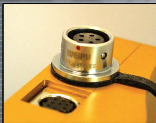
External trigger - Support multiple device, synced video/image grabbing, time-elapsd imaging.
