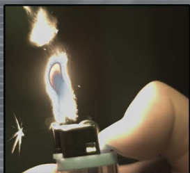
Capturing the moment - ORIA is capable of capturing at 0.32ms of shutter speed, while shooting 150 frames per second. All images are streamed in real-time to a host PC for application-specific processing.
